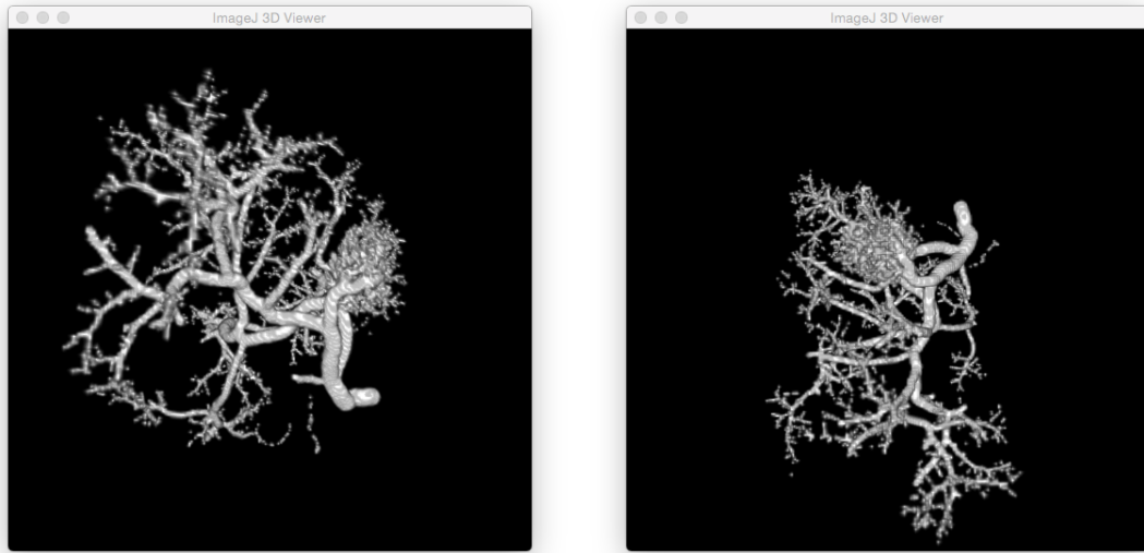
Figure 5.12: Example of complex vascular structures where the parallelised LBM simulation could simulate blood flow. The diameter of the smallest vessels in the presented geometry is 0.5 mm
