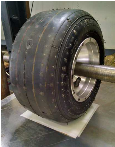
Figure 2.25 – Measurement of contact area of the tyre loaded onto a flat surface using Fuji paper.
