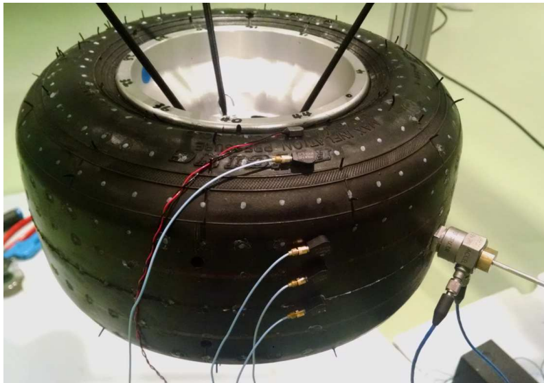
Figure 2.5 – Impedance head and accelerometers mounted onto the suspended reduced-sized tyre.
