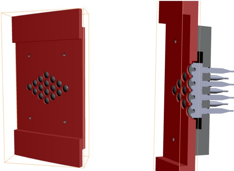
(a) Global view of the rolling surface on the metallic plate hosting multiple asperities. (b) Zoom of the connection between the asperities and the force transducers.
