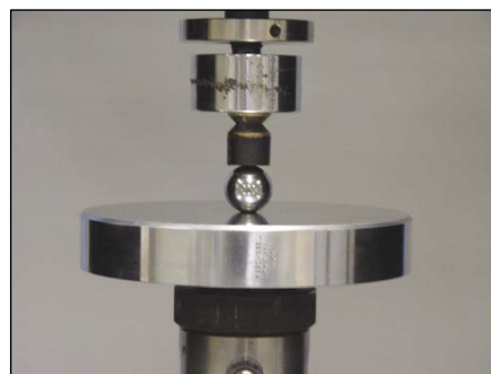
Figure 1.27 – Compress of a rubber pad on a spherical indenter for evaluation of the constant c in equation (1.23) [Sameur, 2004].
