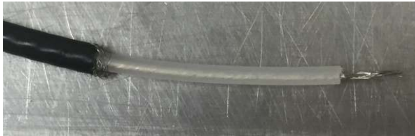
Figure I.20: Sensor based on coaxial cable
