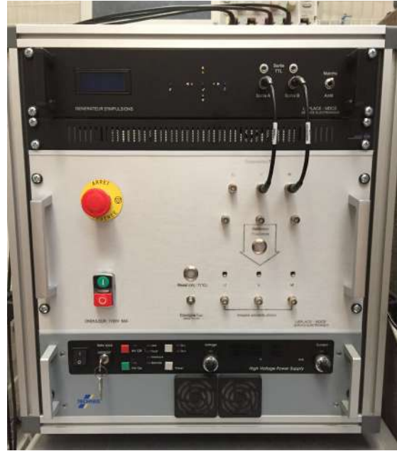
Figure I.21: PWM power supply and command
