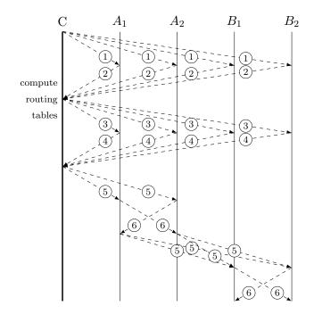
Figure 2.10: Reconfiguration protocol, forwarding routing tables and key states between POIs.
