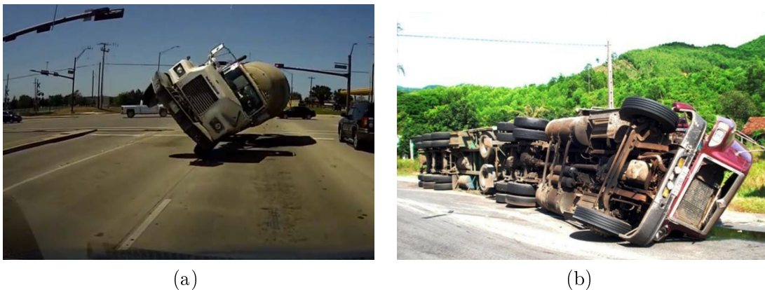
Figure 1.1: Rollover of (a) a single unit heavy vehicle [Carcrushing], (b) a long combination vehicle [Baogialai].
