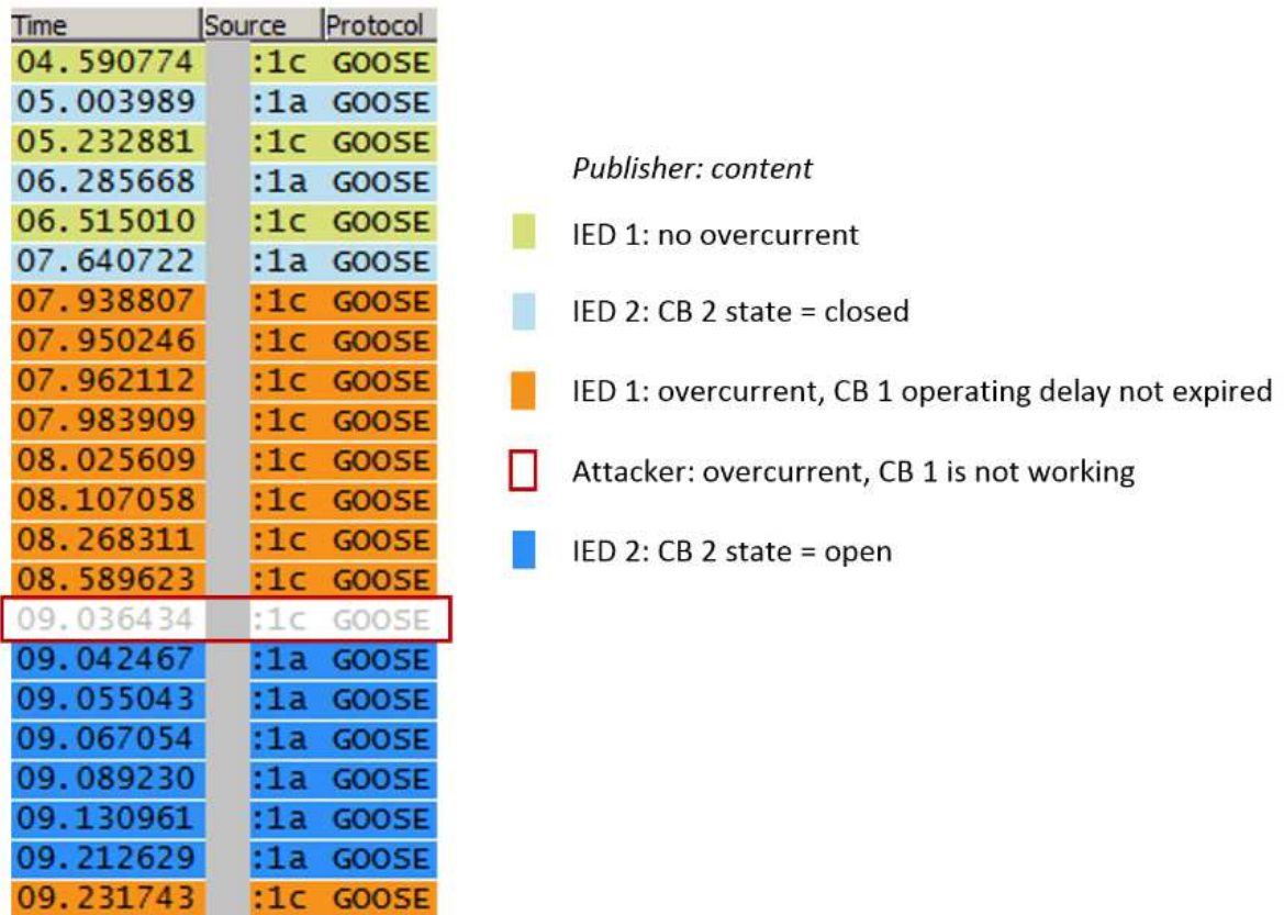
Figure 4.6: Wireshark capture of the GOOSE traffic during attack scenario
