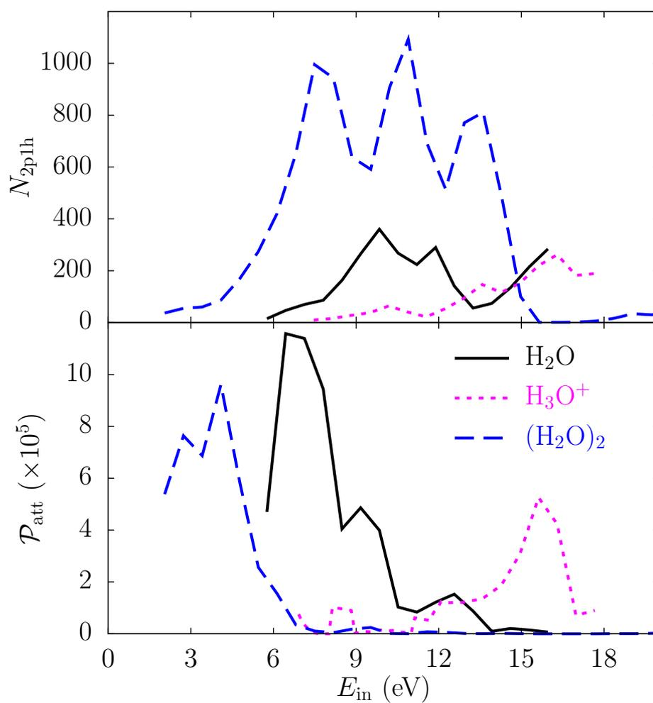
Figure 3.9: Number of  $2p1h$  excitations  $N_{2p1h}$  (top) and asymptotic value of the electron attachment probability  $\mathcal{P}_{\text{att}}$  (bottom) as functions of initial kinetic energy  $E_{\text{in}}$  of the incoming electron, on  $\text{H}_2\text{O}$  (full curves),  $(\text{H}_2\text{O})_2$  (long dashes) and  $\text{H}_3\text{O}^+$  (short dashes). For the sake of clarity, the probability of attachment to  $\text{H}_3\text{O}^+$  has been multiplied by 2.
