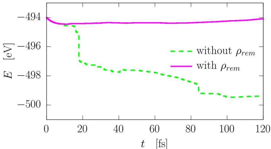
Figure 2.3: Example of discontinuities in the total energy  $E$  in a time evolution of a system (presented in chapter 5) propagated in the Collisional TDHF scheme, with  $\rho_{\text{rem}}$  (solid magenta curve) and without it (green dashes).
