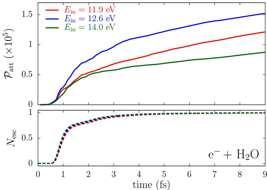
Figure 3.4: Probability of attachment  $\mathcal{P}_{\text{att}}$  (top) defined in Eq. (3.8) and total ionization  $N_{\text{esc}}$  (bottom) defined in Eq. (3.5), as functions of time, for an incoming electron of initial kinetic energy  $E_{\text{in}}$  colliding with a water molecule, at vanishing impact parameter, and for three values of  $E_{\text{in}}$  as indicated.
