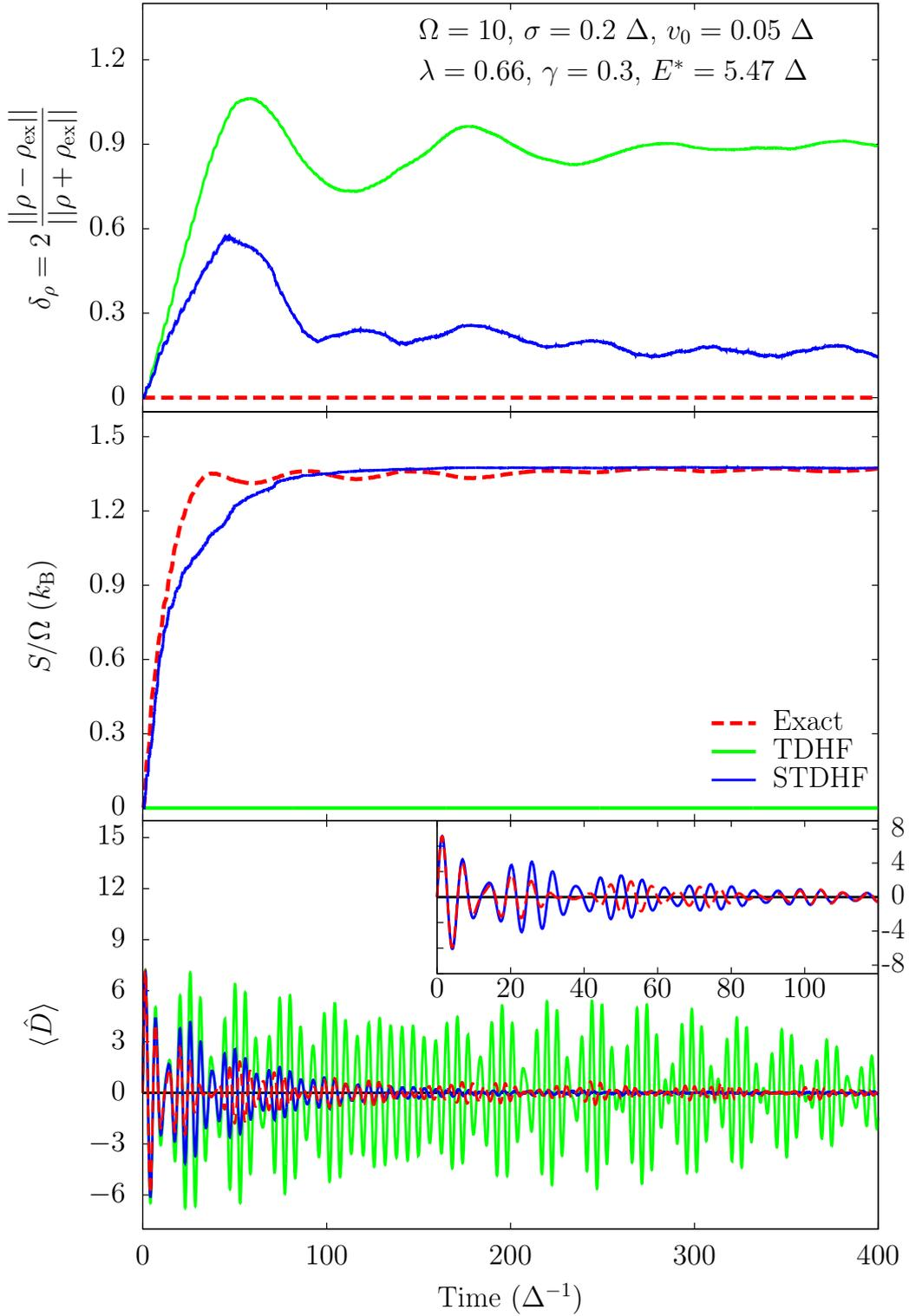
Figure 4.3: Comparison of TDHF, STDHF and exact solution with respect to three observables, as a function of time, with the STBM parameters as indicated. Bottom : expectation value of the dipole operator  $\hat{D}$ , see Eq. (4.15b); middle : entropy per particle  $S/\Omega$ , see Eq. (4.16); top : difference of one-body density.
