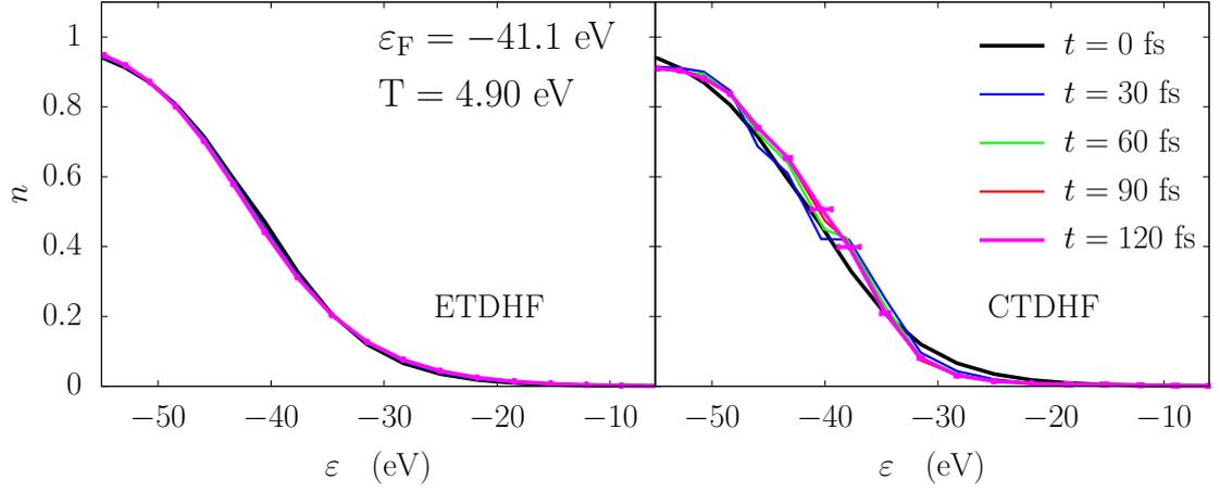
Figure 5.3: Time evolution of occupation numbers starting from a thermal state in ETDHF (left), and CTDHF (right). Quantum error bars are displayed in both cases at final time  $t = 120$  fs but are not visible in ETDHF calculation.
