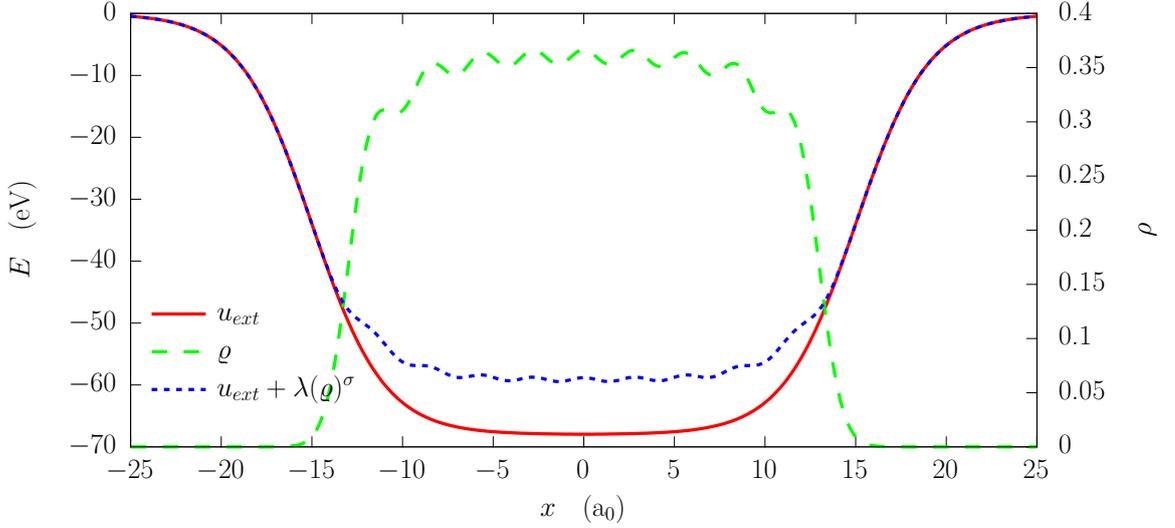
Figure 5.1: External potential coined “1” (red and left vertical scale), ground state density (green dashes and right vertical scale) and full potential (blue dots) plotted against  $x$  in the 1D model.
