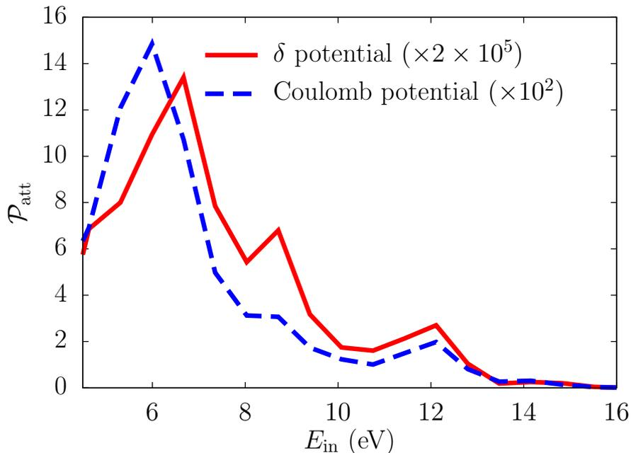
Figure 3.7: Asymptotic probability of attachment to  $\text{H}_2\text{O}$  as a function of energy of incoming electron  $E_{\text{in}}$  for two modeling of  $V_{\text{res}}$ : (red full line)  $\delta$  function or (blue dashed line) the Coulomb potential.
