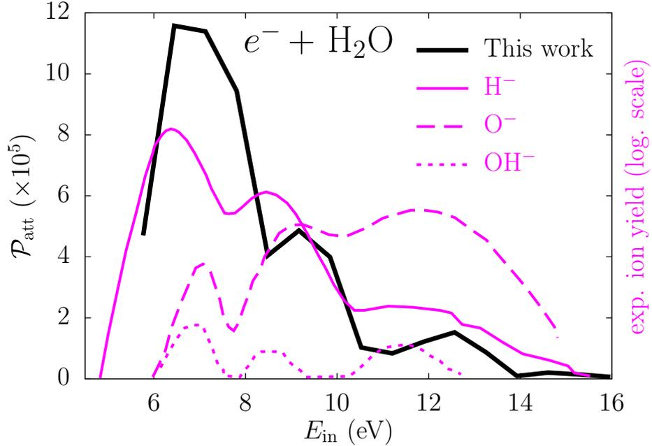
Figure 3.6: Electron attachment to  $\text{H}_2\text{O}$  as a function of energy of incoming electron  $E_{\text{in}}$ . Black thick line and left (linear) vertical scale : asymptotic value of the calculated probability of electron attachment  $\mathcal{P}_{\text{att}}$ . Light curves and right (logarithmic) vertical scale : experimental measurements of dissociative electron attachment yielding  $\text{H}^-$  (solid curve)  $\text{O}^-$  (dashes), and  $\text{OH}^-$  (dots) from [91].
