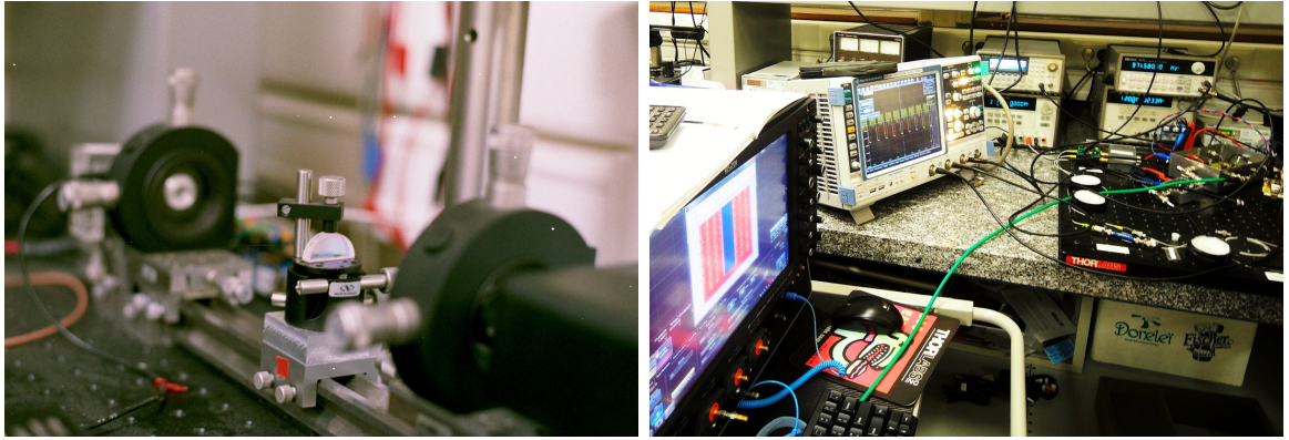
Figure 2.2.10: The experimental setup. Left: The Fabry-Pérot interferometer between the laser and photodetector. Right: The live setup that demonstrates chimera waveforms on each display of the two oscilloscopes.
