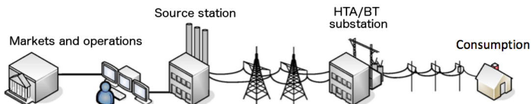
Figure 6.1 – Simplified view of a power grid
