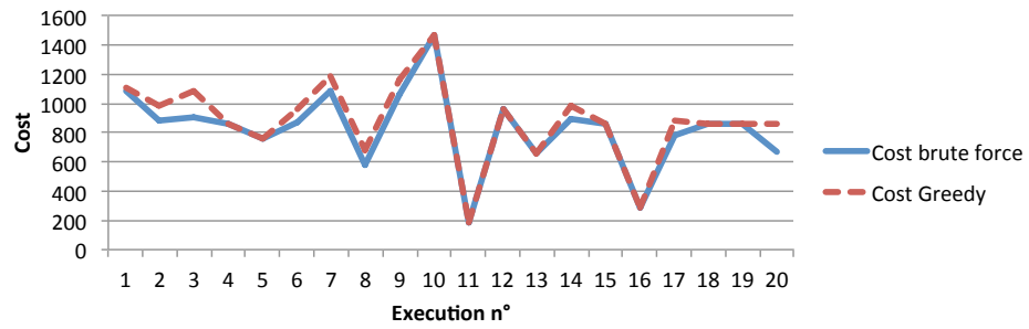
Figure A.2 – Cost of operator mapping: comparison between brute force and greedy algorithm
