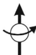
Figure I.2 : Free unpaired electron with a spin angular momentum (curved arrow) and magnetic moment (vertical arrow).
