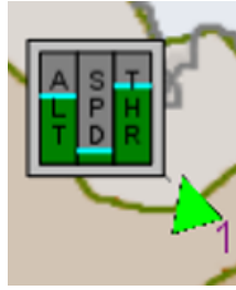
Figure 4.8: Visualisation of the UAV with a medium LOD of the states subsystem - illustrating the graphical aggregation of the UAV states information
