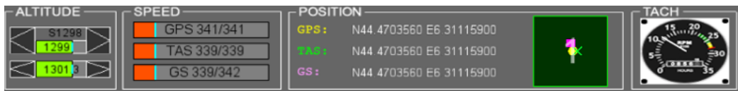
Figure 4.9: Visualisation of the UAV with a low LOD of the states subsystem - illustrating an raw level of UAV states information
