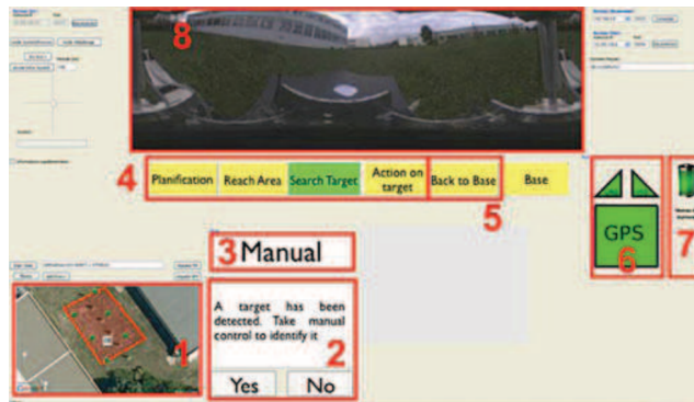
Figure 2.8: Example GCS interface, where (8) illustrates the panoramic view captured by multiple cameras (Published in [187])
