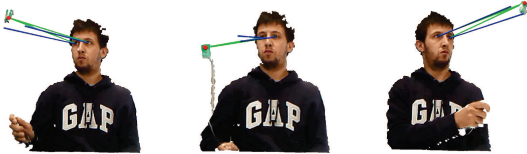
Figure 4.15: Some results of the final gaze estimation using our feature-based system. The green lines define the ground truth and blue lines represent the estimation, the red point shows the tracked object.
