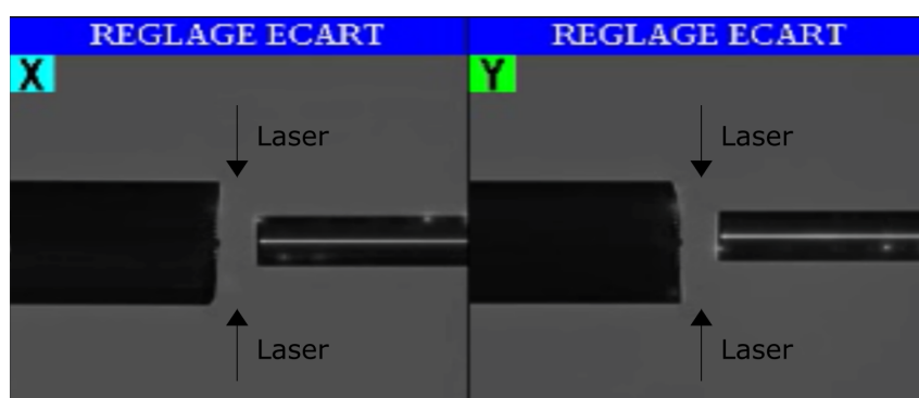
Figure 6.1: Image of the fibers during the splicing process. The cameras in the machine ensure two lateral views of the fibers during the splicing.
