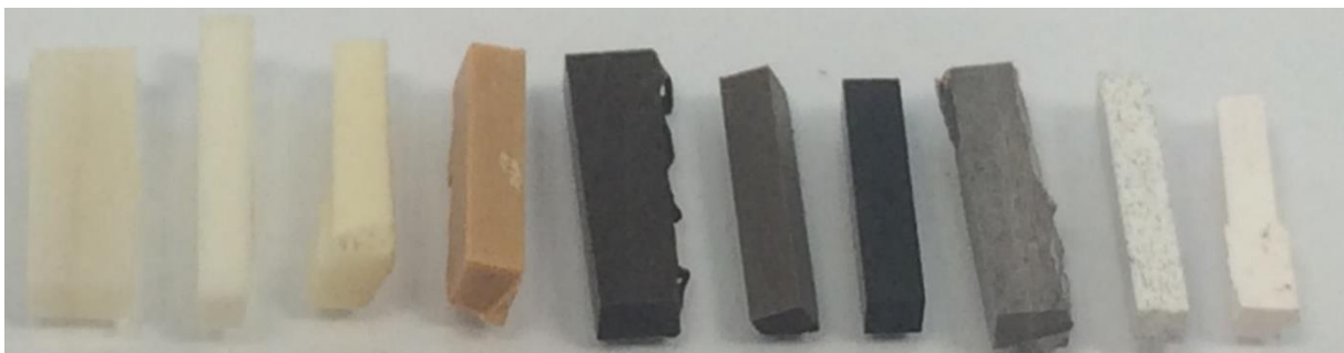
Figure 3.14. Heat treated bovine cortical bone samples for ACOM-TEM. From right to left: control, 100, 150, 200, 300, 400, 600, 700, 800, 1000 °C.
