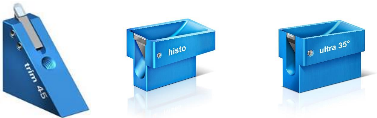
Figure A.1. Diamond knives used in ultramicrotomy. From left to right: trimming knife, histo (semi-thin sections 10 um -150 nm), ultra 35° (ultrathin sections 100-10 nm).
