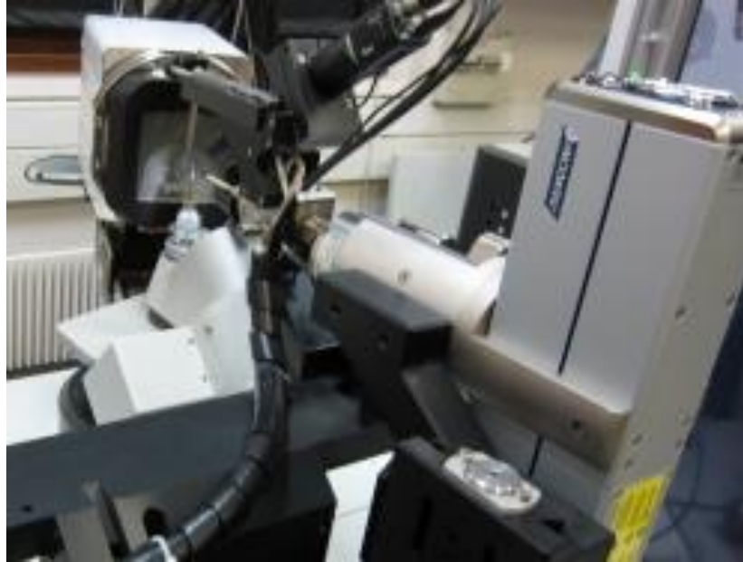
Figure 2.18. Laboratory XRD setup (Institute Neel).
