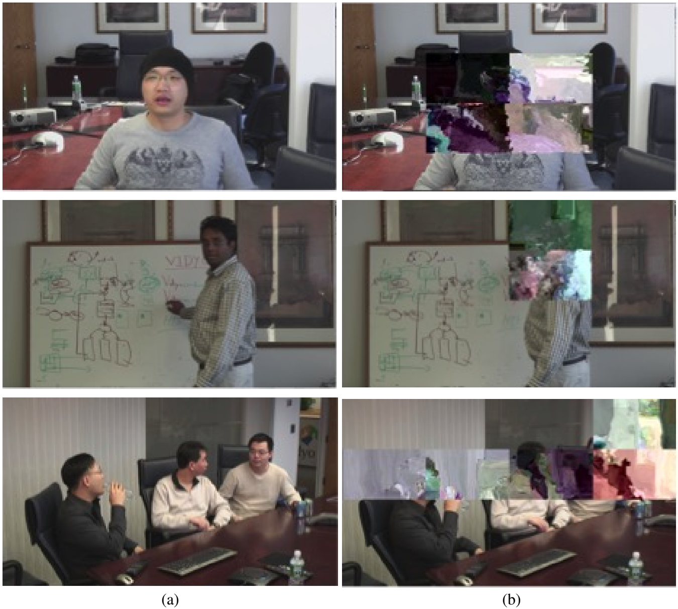
Figure 4.8 – Frame #9 of HEVC videos encrypted with the proposed ROI encryption: (a) Correctly decrypted videos. (b) Encrypted videos.
