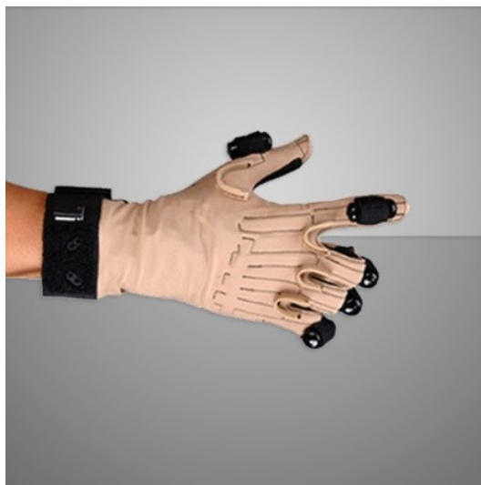
FIGURE 1.24 – Le CyberTouch, CYBER GLOVES SYSTEMS [2016]
