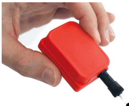
FIGURE 1.20 – La centrale inertielle MTx, XSENS [2016]
