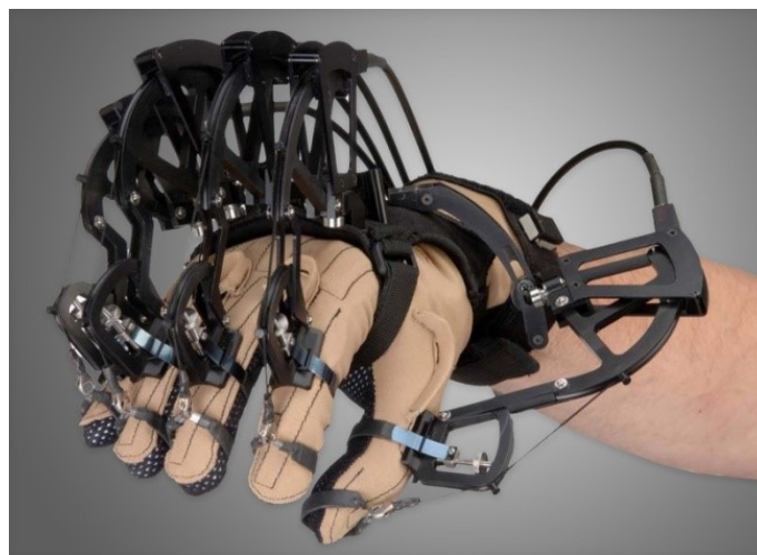
FIGURE 1.23 – Le CyberGrasp, CYBER GLOVES SYSTEMS [2016]
