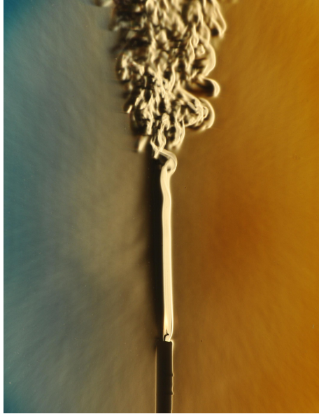
Figure 1.3: Transition to turbulence of the plume of smoke rising from a candle generated by Kelvin-Helmholtz instability.
