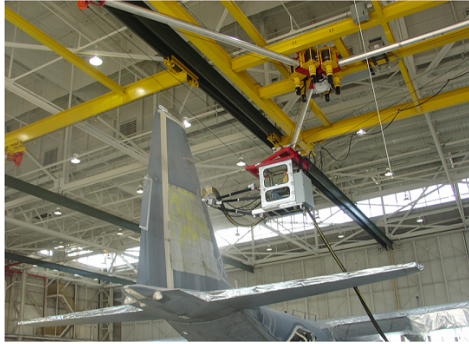
Fig. 1.5 – NIST RoboCrane painting an aeroplane [ ABD92 , ABJ03 ]
