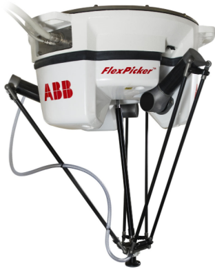
Fig. 1.2 – FlexPicker, a Delta parallel robot from ABB company [ ABB ]
