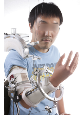
Fig. 1.12 – CAREX, a cable-driven arm exoskeleton [MA12]
