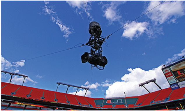
Fig. 1.11 – Skycam, a CDPR for broadcasting of sport events [Sky]
