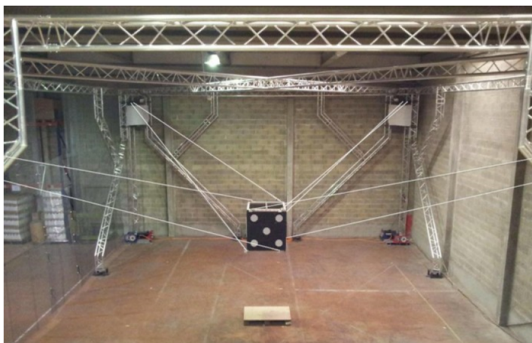
Fig. 1.7 – CoGiRo prototype, designed by the LIRMM and Tecnia [ Pro ]
