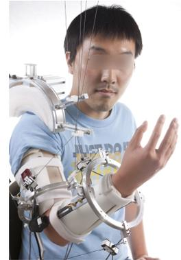
**Fig. 1.12** – CAREX, a cable-driven arm exoskeleton [MA12]
