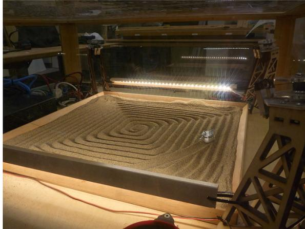
**Fig. 1.15** – Four-Cable Drawing Machine by David Bynoe [Fou]
