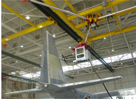
Fig. 1.5 – NIST RoboCrane painting an aeroplane [ ABD92 , ABJ03 ]
