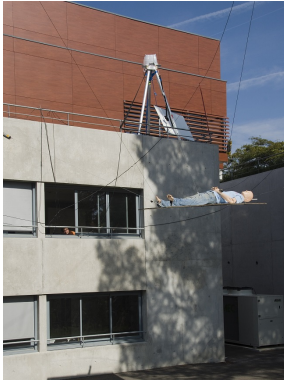
Fig. 1.13 – MARIONET-CRANE during a search and rescue simulation [Mer08, MD10]
