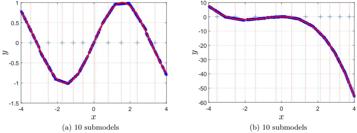
Figure 4.6: PWA modeling of static nonlinear functions from noise-free data: observations (black dots); true nonlinear function (red solid line); PWA function (blue stars). The crosses indicate the positions of the centers  $\{c_i\}$ .
