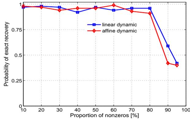
Figure 2.4: Estimates of probabilities of exact recovery by reweighted  $\ell_1$  minimization when noise  $\{e_t\}$  is equal to zero. Results of a Monte-Carlo simulation of size 100 with randomly generated linear ARX systems with orders  $n_a = n_b = 2$ .
