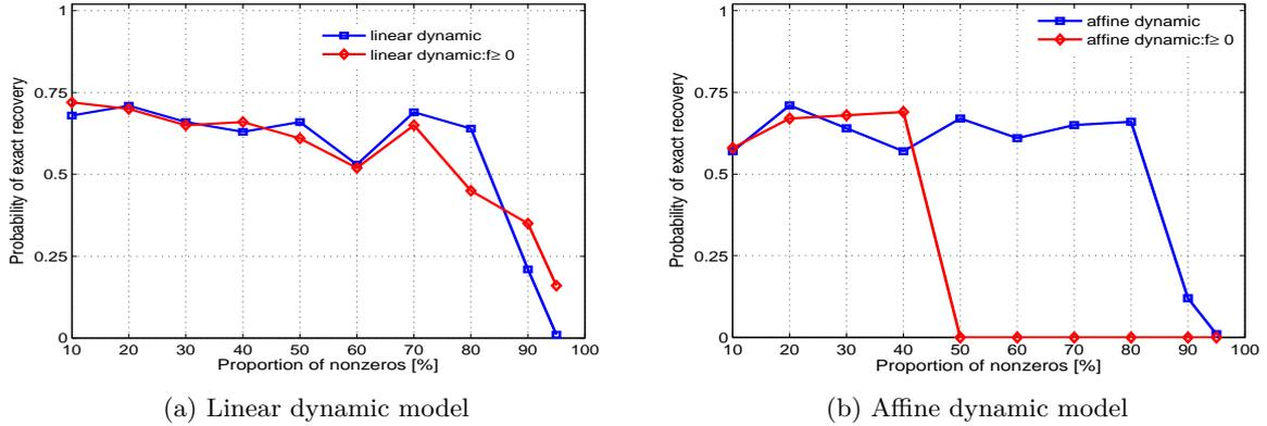
Figure 2.3: Estimates of probabilities of exact recovery when noise  $\{e_t\}$  is equal to zero. Results of a Monte-Carlo simulation of size 100 with randomly generated linear ARX systems of order  $n_a = n_b = 2$ .
