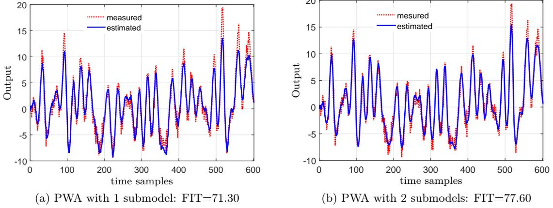
Figure 4.8: PWA modeling of a nonlinear system: comparison of system and model outputs. The model is identified with 60% of the data and validation is done on the entire data set.
