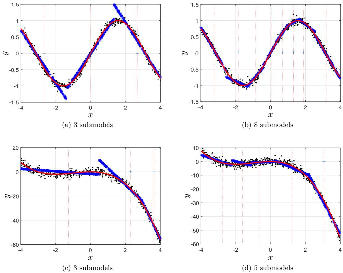
Figure 4.5: PWA modeling of static nonlinear functions from noisy data with the proportion of noise being such that the SNR is equal to 20 dB: noisy data (black dots); true nonlinear function (red solid line); PWA function (blue stars). The two top subfigures are related to system (4.41) while the two other pertain to system (4.42).
