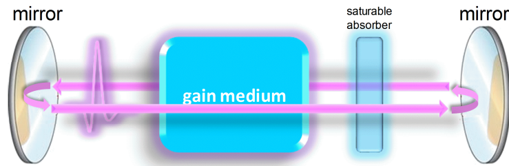
Fig 3.14 | Experimental setup for passive mode-locking by inserting a saturable absorber inside the laser cavity.
