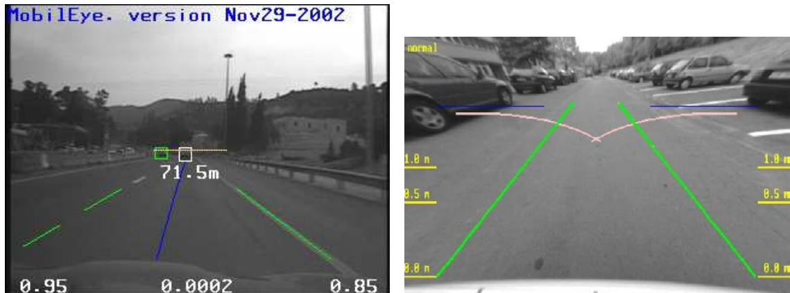
(a) Front view with lane and object detection for longitudinal control, lane keeping, collision mitigation, collision avoidance, etc. Image: [46]. (b) Rear view for parking aid and collision avoidance, collision avoidance, etc. Image: [46].
