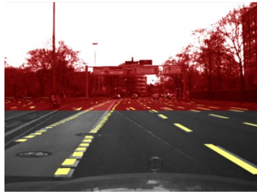
(d) This figure demonstrates the matching result after 10 iterations of the ICP algorithm
