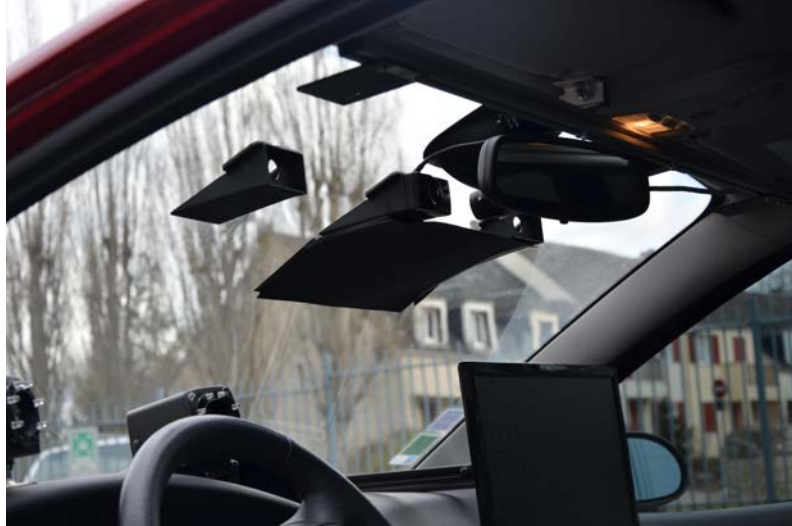
Figure 2.19: LDWS camera utilized in this thesis. The camera is forward looking and located behind the windscreen.
