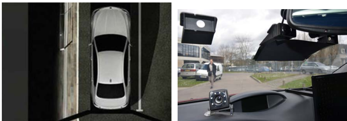
(c) Surround view for parking and maneuvering. Image: [55]. (d) Interior view for driver drowsiness monitoring aid. Image: [55].
