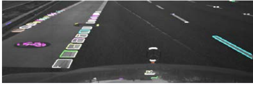
(a) The authors used Canny edge detection to cluster the lane marking feature
