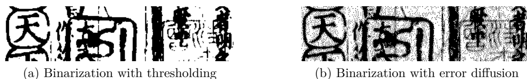
Figure 4.3.1: Comparison of thresholding and error diffusion binarization techniques.
