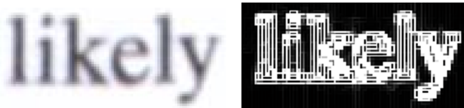
Figure 5.5.4: CCC segmentation and color distance map produced by Watercolor. Left: each region has a uniform color. Right: the pixel intensity represents the distance value. Notice the vertical rectangles in the “l” characters. The white borders will produce several regions.
