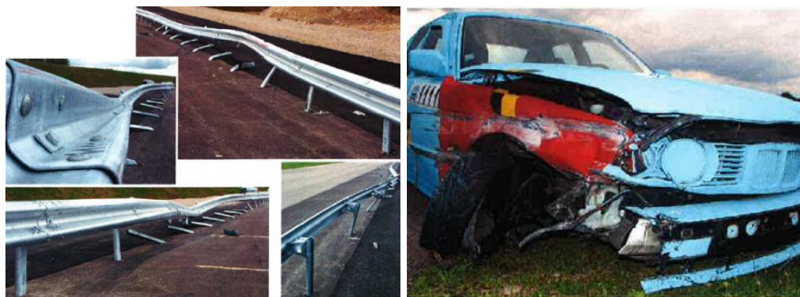
Figure 3- 6 Damage of the barrier and vehicle [60]
