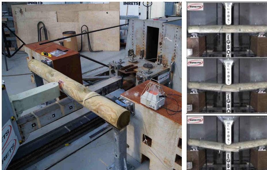
Figure 2- 7 Bending test of steel reinforced wood beam [49]
