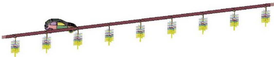
Figure 1- 19 Boundary constraints' simplifications of the VRS with spring elements [15]
