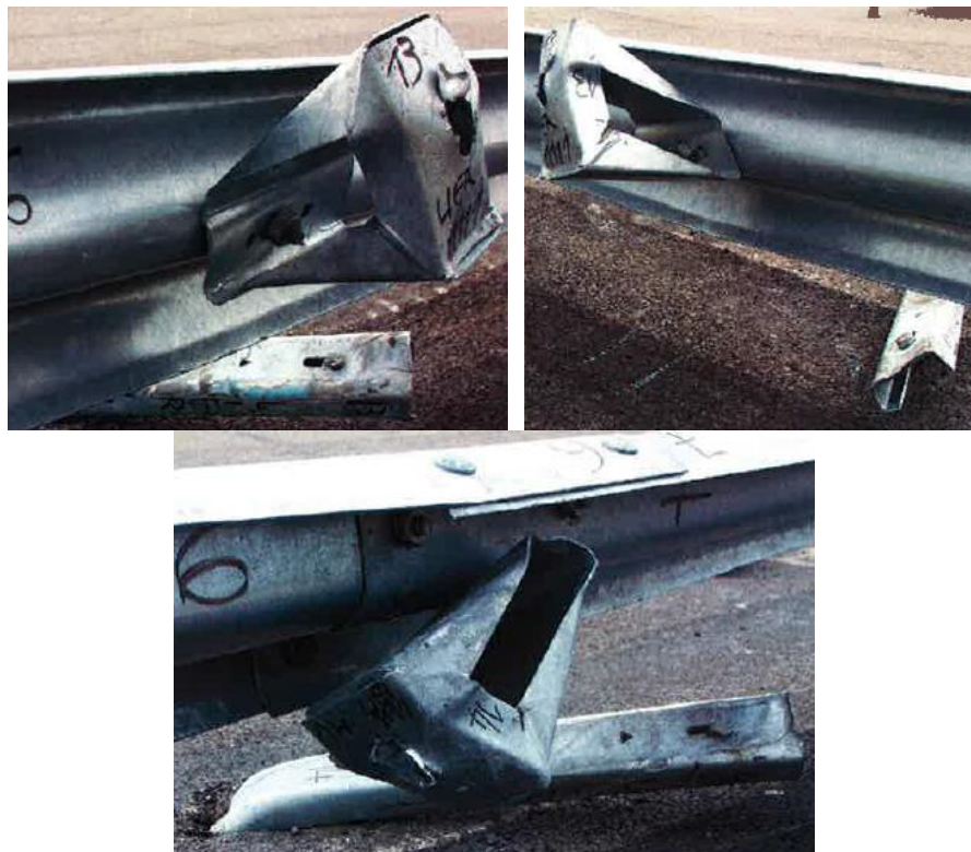
Figure 3- 18 Bolts pull out failure of post-spacer connection [60]
