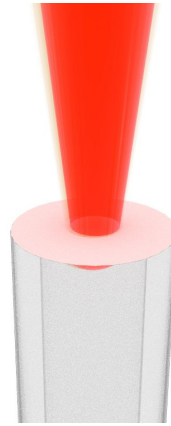
Figure 3.6 – Principle of laser ablation : a CO 2 laser is highly absorbed in the first tens of microns of silica.
