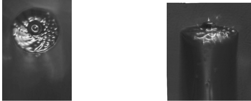
Figure 3.17 – A “pencil” shape fibers observed with a microscope. the rough surface far from the mirror reflects the shooting pattern .The diameter of the fiber is 125\ \mu\text{m} , the concave depression RoC is 10\ \mu\text{m} . SEM image of such a fiber is displayed on the front page of this chapter.
