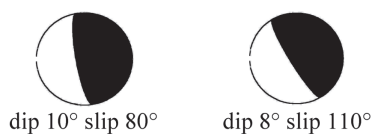
Fig. 3 Focal mechanisms of the 1960 Chilean earthquake (left) and of the 2004 Sumatra event (right).
