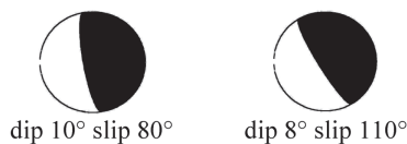
Fig. 3 Focal mechanisms of the 1960 Chilean earthquake (left) and of the 2004 Sumatra event (right).
