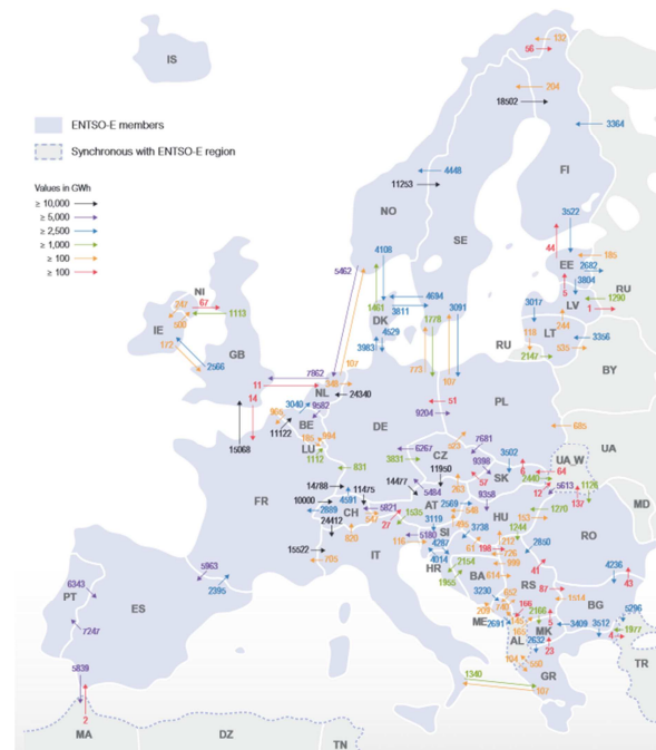
Figure I-4 - Physical energy flow values in GWh in 2014 in the ENTSO-E area [ENTS-15]
