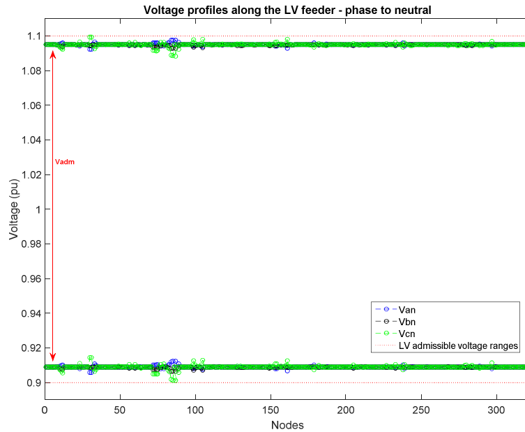
Figure AIV-6 – Voltage profiles of the LV ESR network with the summer loading case and determination of the new MV admissible voltage range
