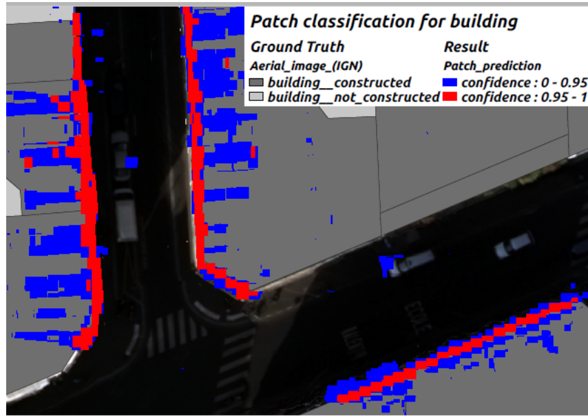
Figure 154: Plotting of patches classified as building, using confidence to increase precision. Ground truth from IGN and Open Data Paris
