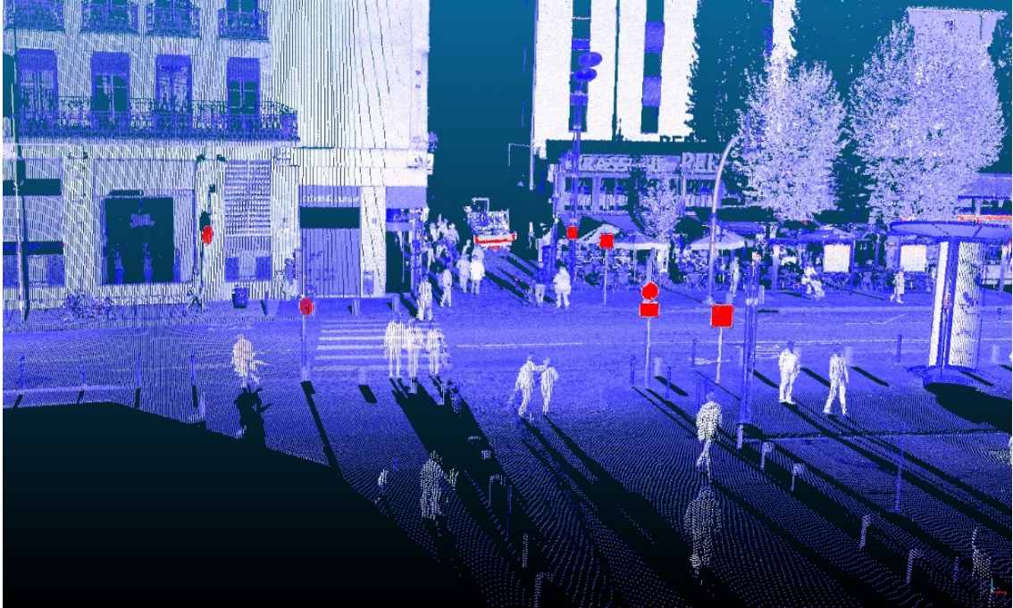
Figure 11: Street Lidar Point cloud ( intensity tone from blue to white to red).
