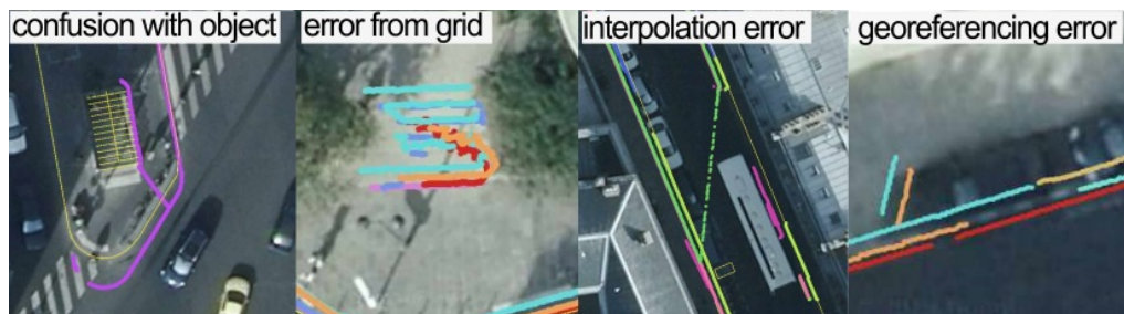
Figure 117: Input kerb detection is consolidated and filtered (both geometrically and with context) to produce more reliable observations.
