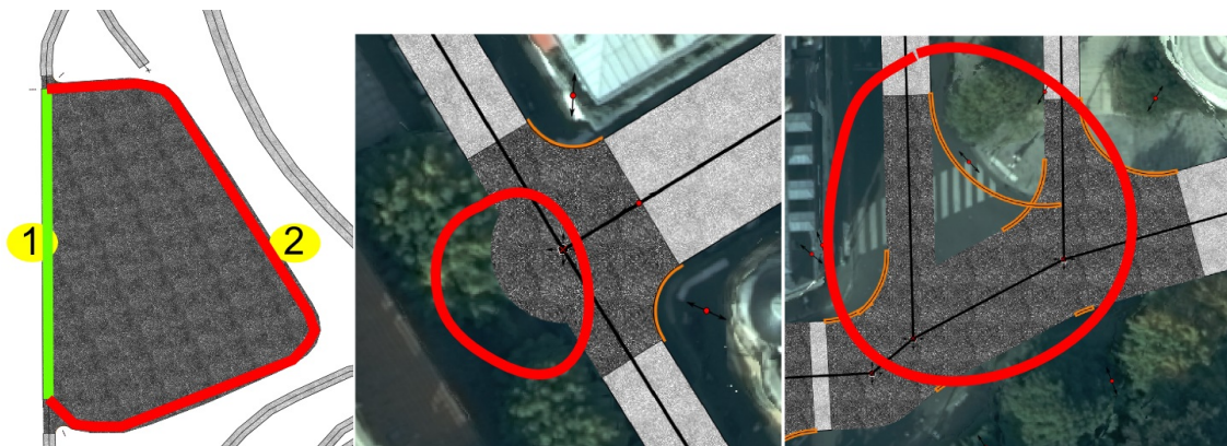
Figure 71: Various cases of failure from more severe to less severe (1 , 2 , 3). 1 : loop, 2 : bad buffer use, 3 : radius too big for network.
