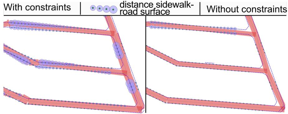
Figure 122: Constraints are necessary to stay close to the initial solution. However, they can significantly degrade the results when there are enough quality observations. Circles are proportional to the distance between ground truth and result. Note that constraint influence can be modulated with weights.
