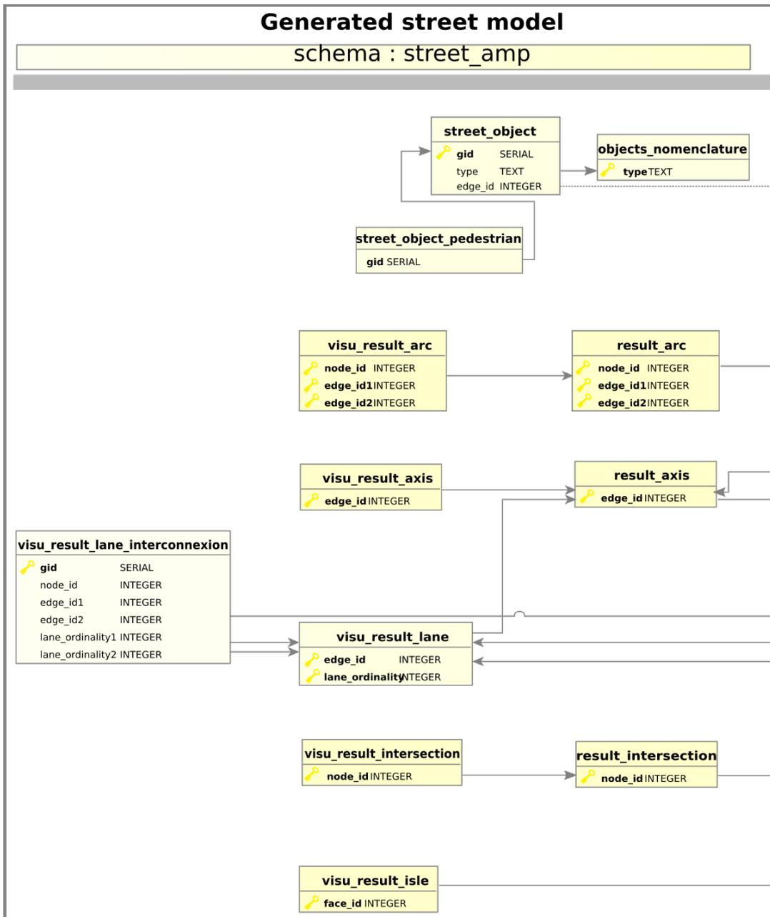
Figure 159: StreetGen base table schema in database (part 1/2)
