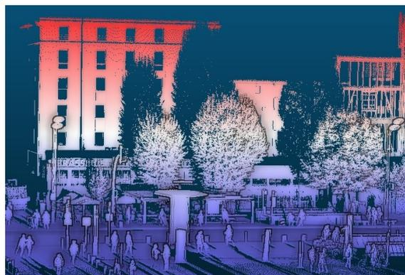
Figure 7: On this street Lidar point cloud, trees are clearly masking building facades, creating occlusion.
