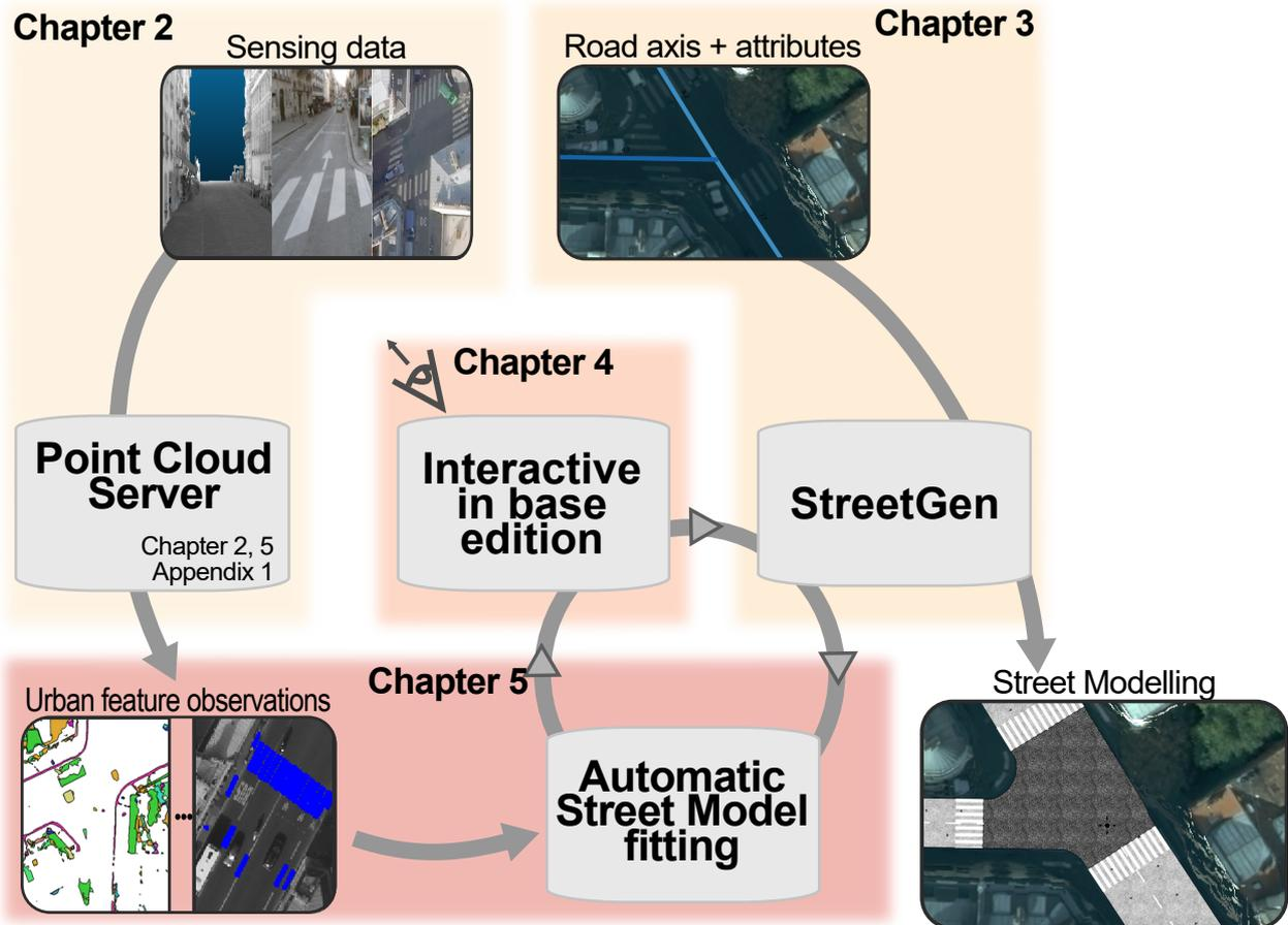
Figure 4: Thesis graphical abstract. From an approximate road axis network a street modelling is generated with StreetGen (Chapter 3). Such modelling is interactively edited with any GIS using Interactive In Base edition (Chapter 4). In complement, the street modelling can be automatically fitted (Chapter 5) to massive sensing data, managed with a Point Cloud Server (Chapter 2, Appendix A) .
