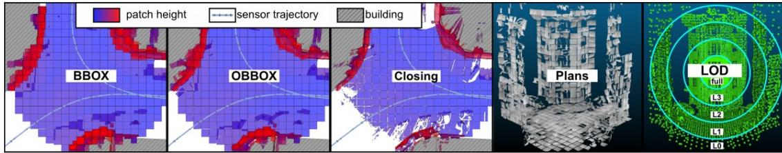
Figure 38: Streets and buildings. Generalisation like Bounding Box, Oriented BBox, Spatial closing. Closing on 3D plan detection. Level Of Details.
