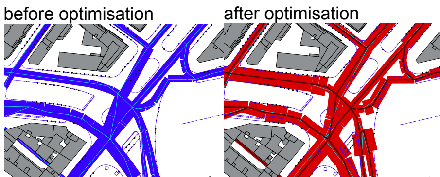
Figure 121: Even in very complex situations, where observations are too sparse and the simple road model is not sufficient, results are stable (no constraints used).
