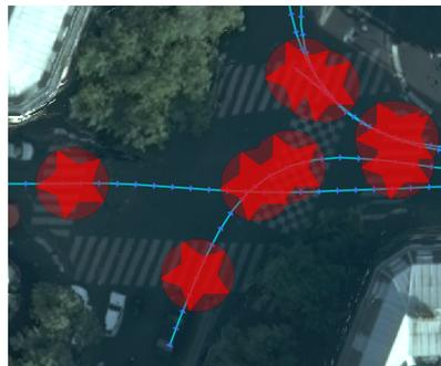
Figure 39: Rough pedestrian crossing detector.
