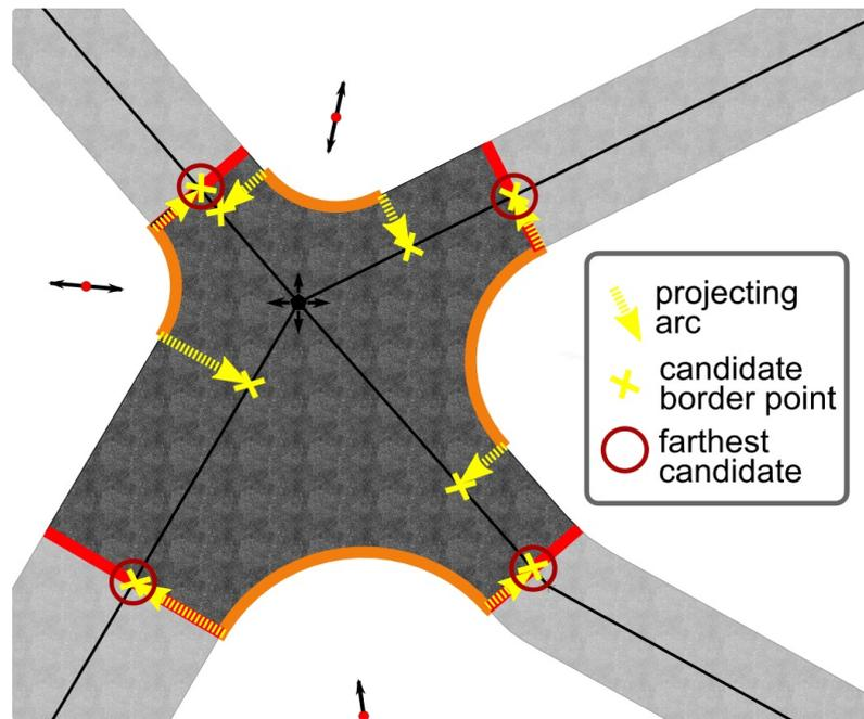
Figure 52: From circle centres, border points that limit the intersection are found by projection and filtering (farthest from intersection centre).
