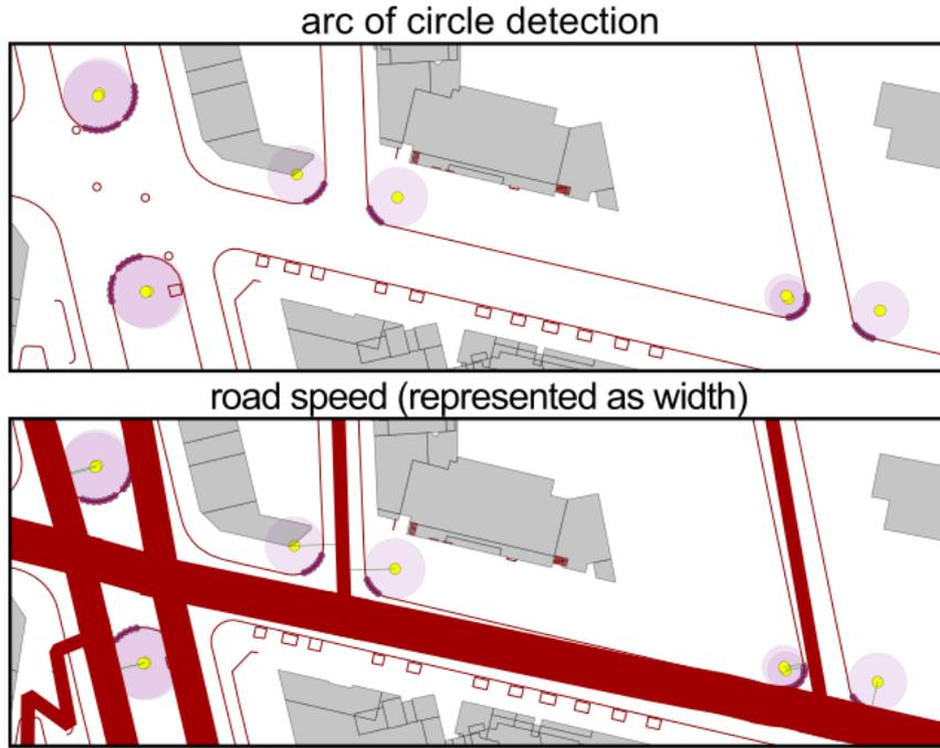
Figure 68: Radius detection and average road speed obtained by various dataset merging.
