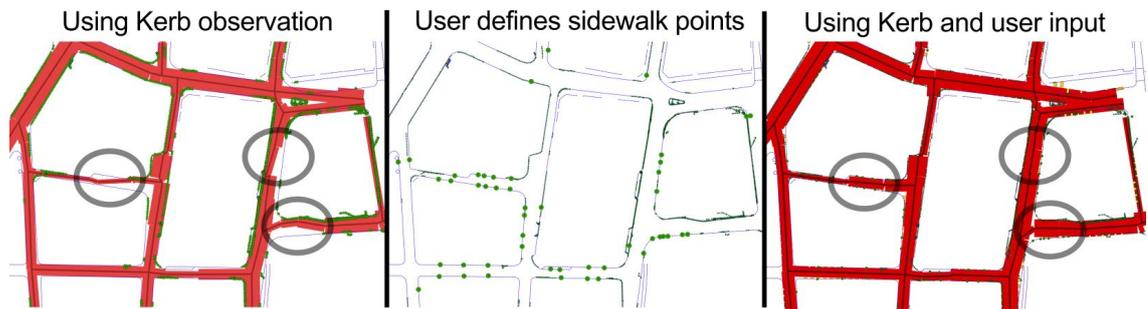
Figure 126: Optimisation results based on kerb observations for "user" experiment area.
