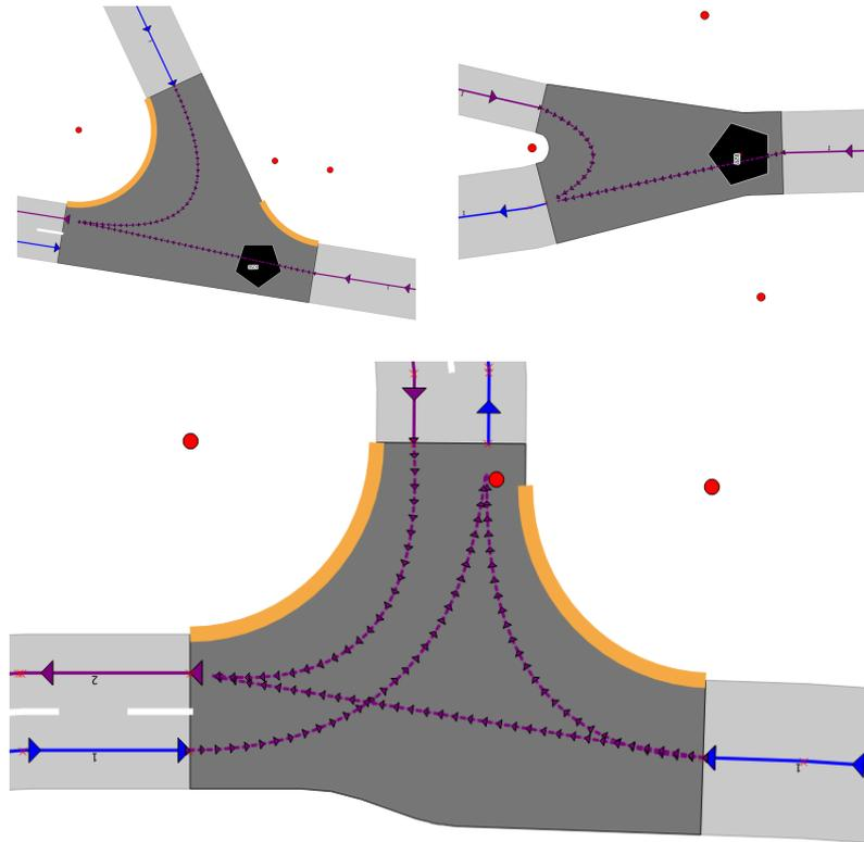
Figure 61: interconnection trajectory, Bezier curve influenced by start/end and possibly intersection centre.
