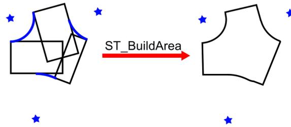
Figure 54: From cutted axis surfaces and arcs, the function `ST_BuildArea` build the maximum area possible.
