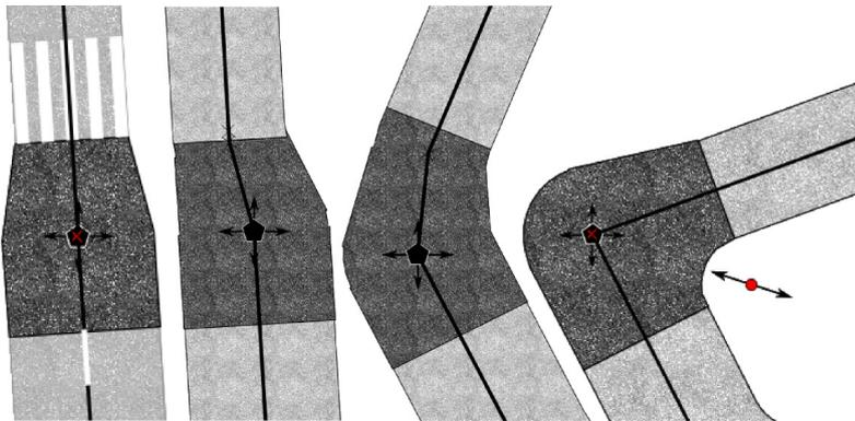
Figure 55: Variable buffer for robust roadway width transition.
