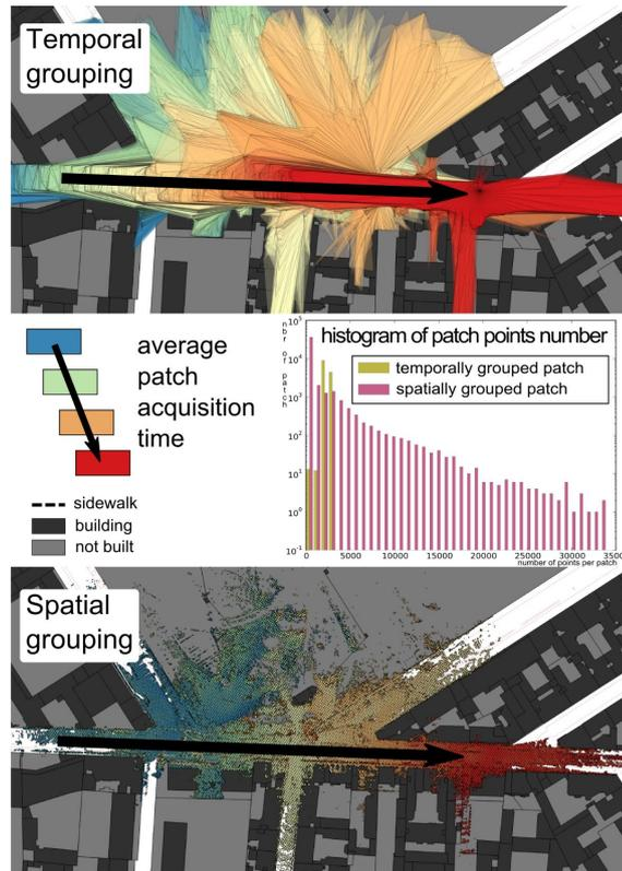
Figure 33: Temporal (left) and 3D spatial (right) grouping on velodyne terrestrial Lidar data, with histogram of number of points per patch. Note that in practice we use mixed grouping (spatio-temporal).
