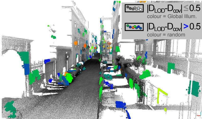
Figure 148:  $\text{Dim}_{\text{LOD}}$  and  $\text{Dim}_{\text{cov}}$  are mostly comparable, except for few patches (5%, coloured)
