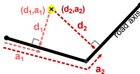
Figure 102: A unique absolute position can correspond to several relative positionings, which theoretically limits relative positioning setting through absolute geometry.
