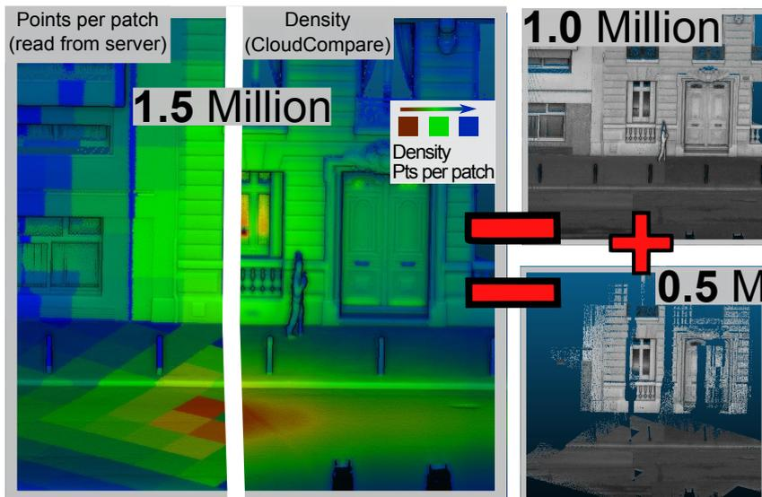
Figure 140: Abnormal density detection and correction. Top points per patch (left) or density (right), green-yellow-red. Bottom reflectance in grey.
