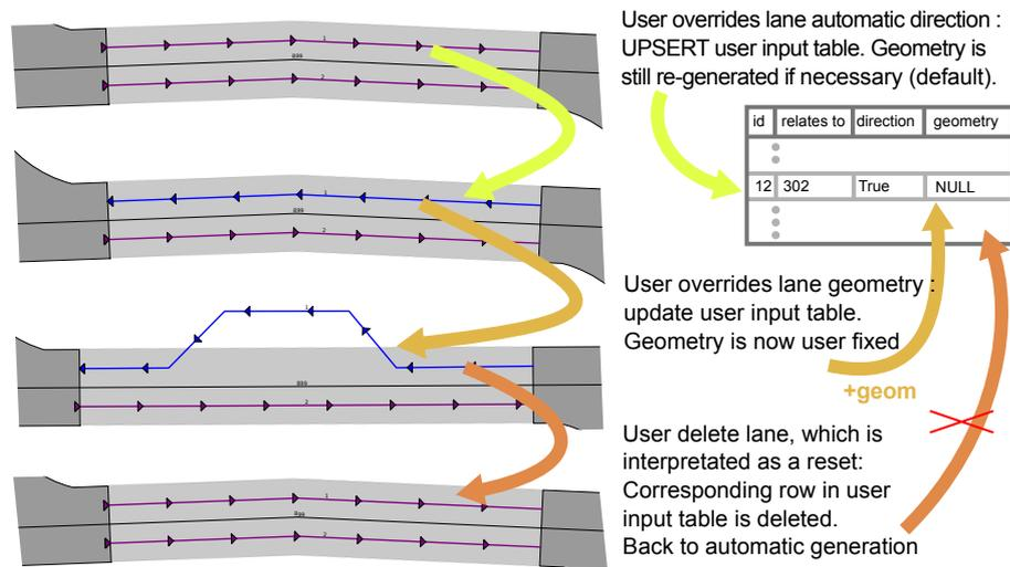
Figure 91: When the user overrides a default behaviour, the parameter is stored in a user input table. Objects overridden do not use default generation anymore thanks to COALESCE. The user can still delete the overridden object to return to the generic behaviour.
