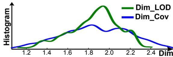
Figure 156: Histogram of  $\text{Dim}_{\text{LOD}}$  and  $\text{Dim}_{\text{cov}}$  for patch in trees (500 kpts). Tree dimension could be from 1.2 to 2.6, yet  $\text{Dim}_{\text{LOD}}$  is less ambiguous than  $\text{Dim}_{\text{cov}}$
