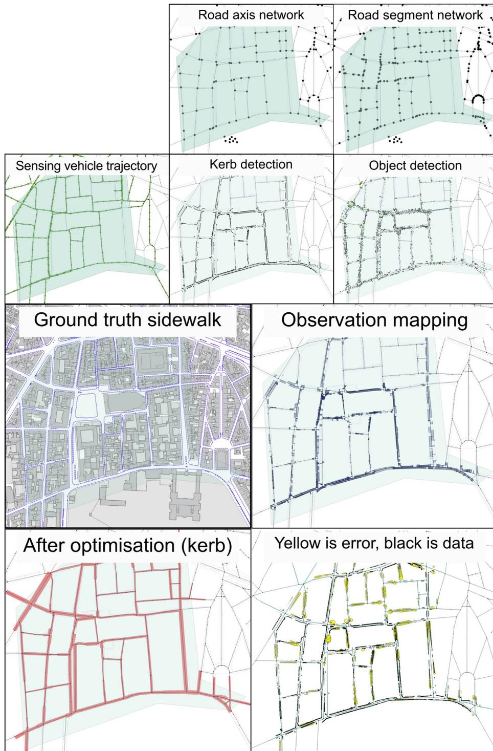
Figure 124: Optimisation parameters are the street axis network and width attribute, which get split into a road segment network. A street sensing vehicle detects kerbs and objects, which are processed into observations, and matched to street segments. Non-linear least square optimisation fits the parameters to these observations.
