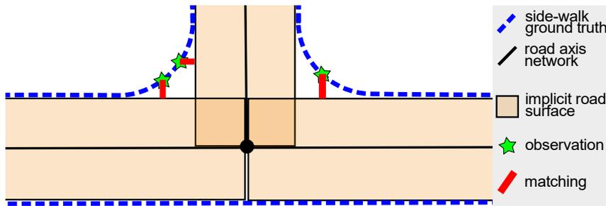
Figure 111: In intersections, kerb observations can not be used as the road model is not adapted. Using these observations would lead to incorrect results.
