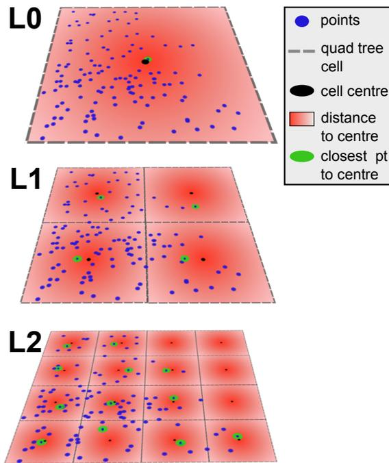
Figure 136: MidOc explained in 2D. Given a point cloud (Blue) and quad tree cells (dashed grey), the chosen point (green ellipse) is the one closest to the centre (black point) of the cell.
