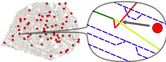
Figure 128: After the optimisation process, the road axis network contains a few topological errors despite the use of constraint forces. These 74 errors for the whole "Paris" experiment area can be corrected by a user in about 10 minutes.
