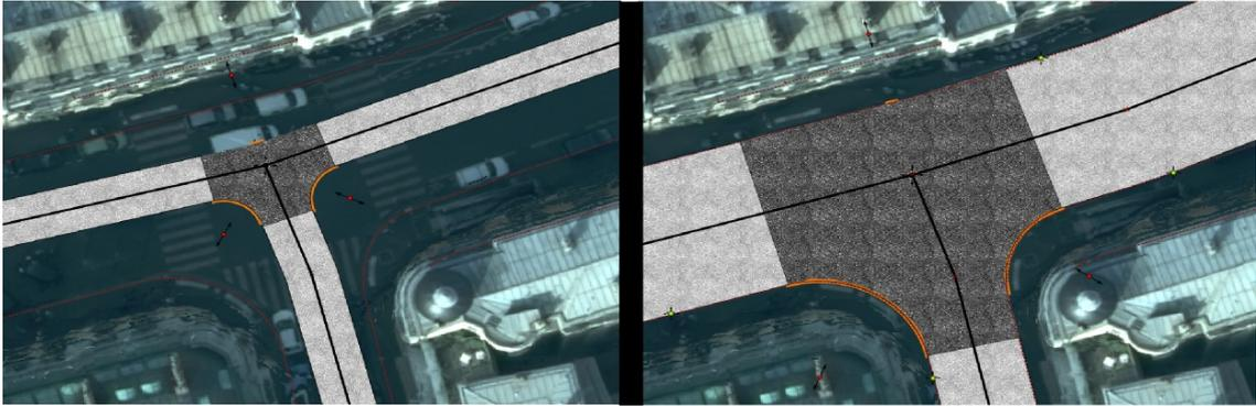
Figure 72: The estimated parameters may be far from reality (Left). It is, however, possible to manually or automatically fit the street model.
