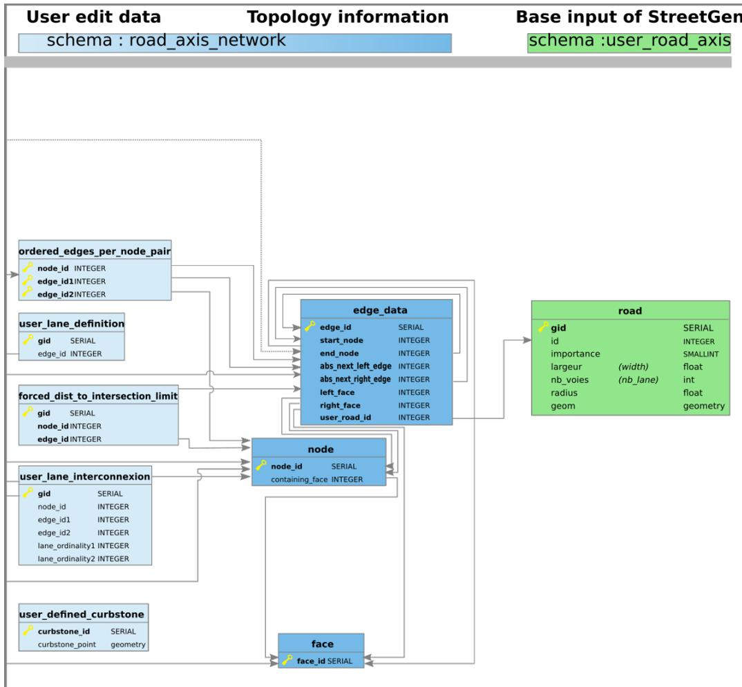
Figure 160: StreetGen base table schema in database (part 2/2)
