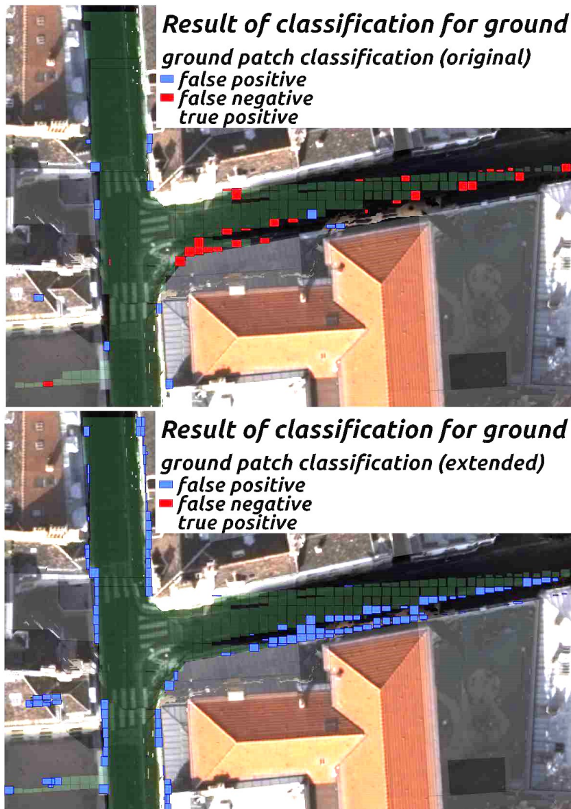
Figure 155: Map of patch clustering result for ground. The classical result finds few extra patches that are not ground (blue), and misses some ground patches (red). Recall is increased by adding to the ground class all patches that are less than 2 meters in X,Y and 0.5 meter in Z around the found patches. Extra patches are much more numerous, but all the ground patches are found.
