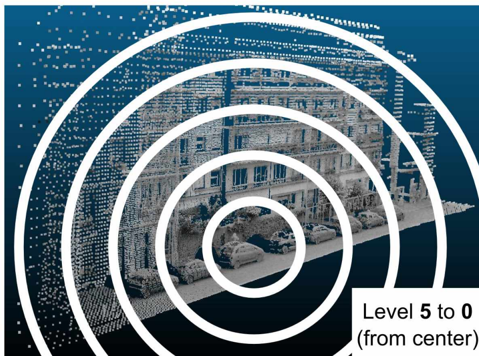
Figure 142: Schematic example of LOD depending on distance to camera
