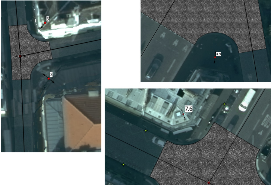
Figure 49: 3 different radius size (3m, 4.9m, 7.6 m) for streets of various importance, from real Paris data
