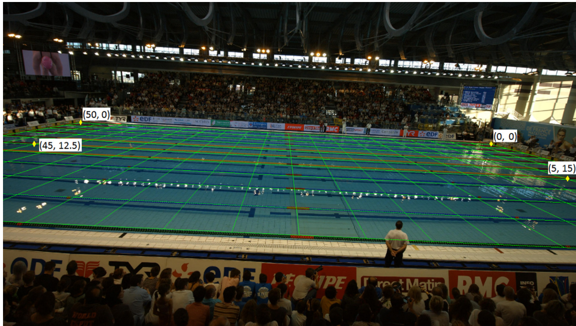
Fig. 1. Swimming pool calibration with the 2D DLT technique after a selection of 4 points. After the calibration, we superimpose a grid of a 50 \times 25 \text{ m}^2 , where the horizontal and the vertical distance between the lines is equal to 2.5 m. (French National Championships, Limoges, April 2015).
