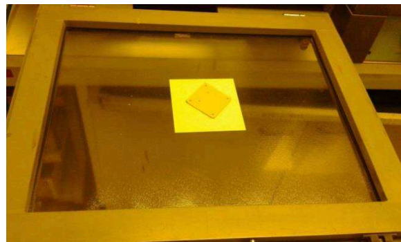
Figure 6. LTCC layer under vacuum to eliminate air between layers
