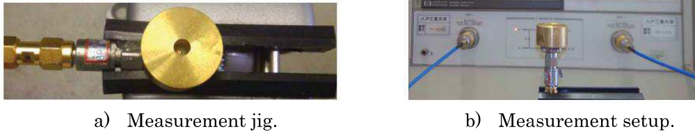
Figure 1.5. Open-ended coaxial line reflection method presented in [5].
