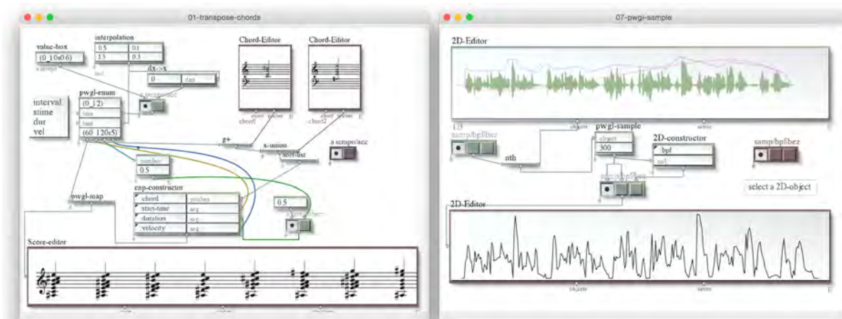
Fig. 1.3: Left: A PWGL patch for transposition of chords. Right: A break point function generated via extraction/resampling of audio data.
