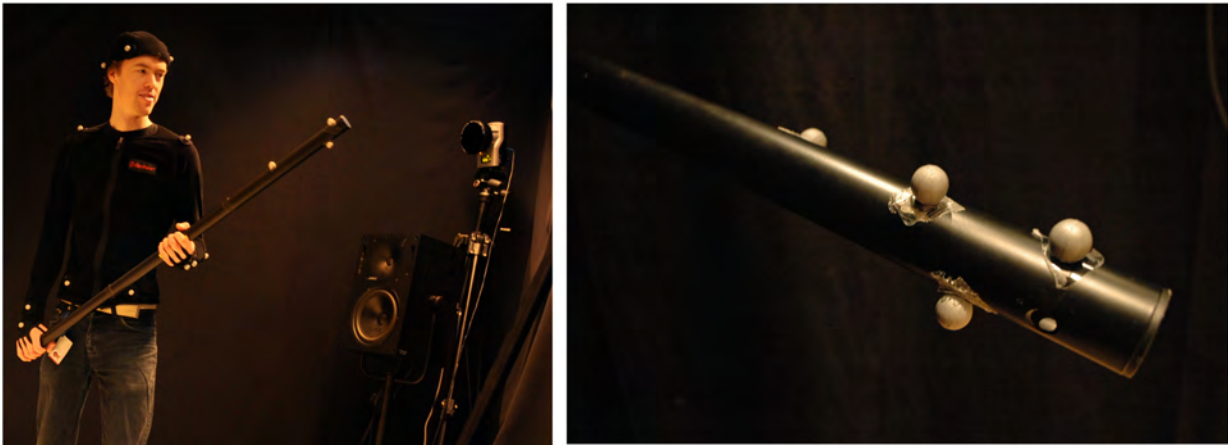
Fig. 3.12: Left: Kristian Nymoen performing with the SoundSaber DMI. Right: close-up of optical markers on the pvc tube. Used with permission.
