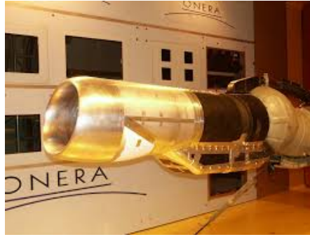
Figure 1.2 – Negatively scarfed intake, picture taken from [81].
