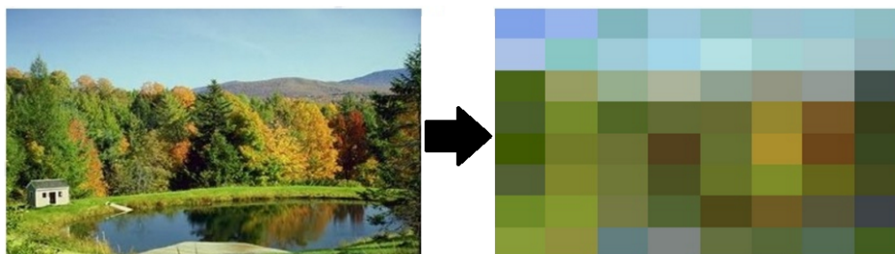
Figure C.1: Color Layout Descriptor. Representative colour selection on a 8 \times 8 partitioned image.
