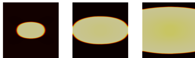
Fig. 3.29: Central stimulus. Standard bidomain model. Observing transmembrane voltage, v at times: 20ms , 50ms and 100ms (left to right).
