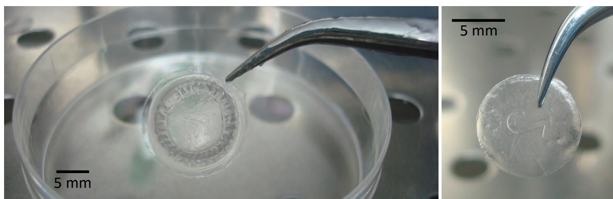
Figure 76. Hybrid collagen-inspired peptide membranes. Left: raw membrane after unmolding. Right: cut membrane.
