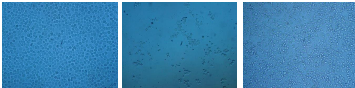
Cell observation after 30 min adhesion and 1h incubation with Prestoblue solution. Left : Tissue culture treated polystyrene; Middle: Hybrid PEG hydrogel without RGD; Right: 20 mol% hybrid RGD hydrogel.
