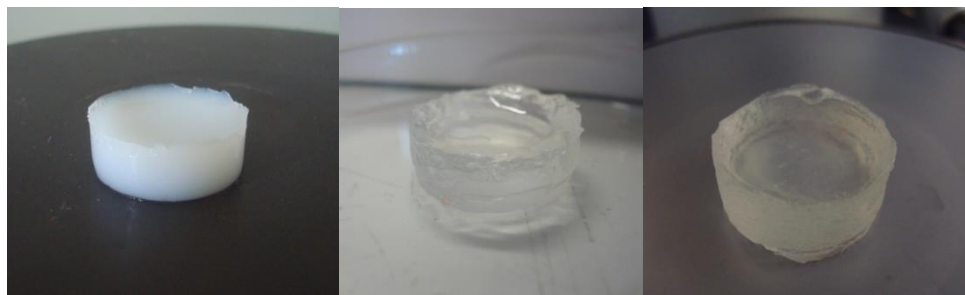
Left: 5 wt% hybrid PEG gel; middle: 10 wt% hybrid PEG gel; right: 20 wt% hybrid PEG gel.
