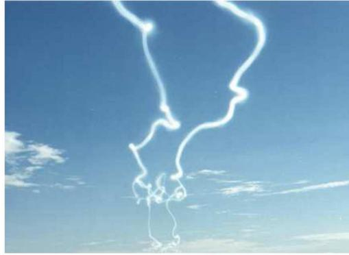
Figure 1.10: Meandering of trailing vortices, from Brion [14].
