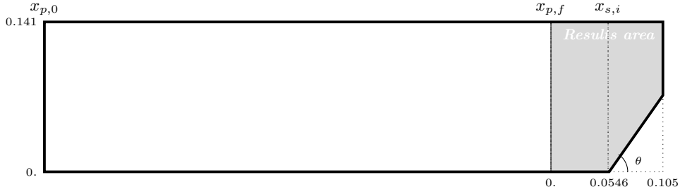
Figure B.12: Schardin's problem configuration with x_{p,0,lag} = -0.475 the initial lagrangian position of the piston, x_{p,f} = 0 . the final position of the piston and x_{s,0} = 0.0536 the position of the incident shock.
