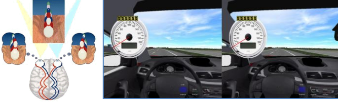
Figure 8: Generation of Dual Screen for 3D immersion based on stereoscopic principle.
