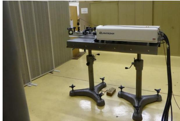
Fig. II.25: Lighting apparatus for the high speed PIV
