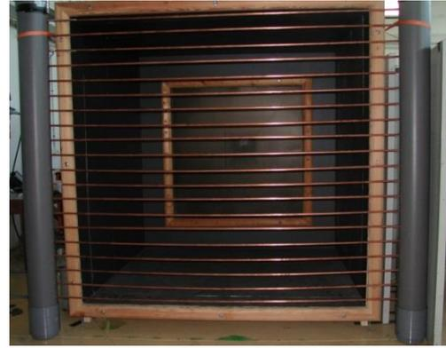
Fig. II.2: Collector and seeding grid
