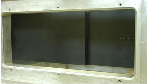
Fig. II.5: Backward facing step in the boundary layer wind tunnel
