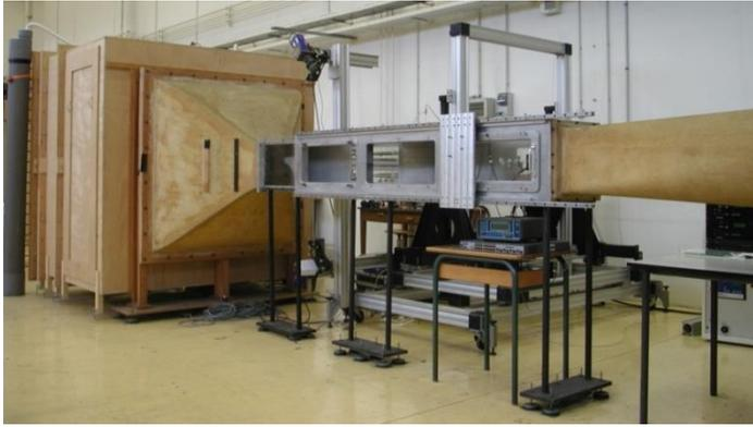
Fig. II.1: Boundary layer wind tunnel
