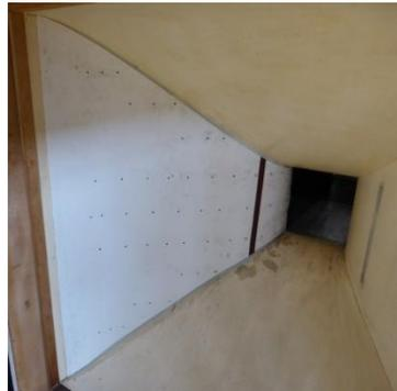
Fig. II.7: Wind tunnel collector modifications
