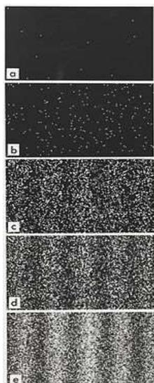
**Figure 16 : Demonstration of single electron build up of an interference pattern**
