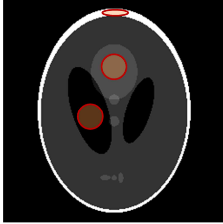
Figure 9: ROIs selected for qualitative assessment on the Shepp-Logan phantom reconstruction. The upper ROI corresponds to bone, the middle ROI to soft tissues (ST) and the bottom ROI to air.
