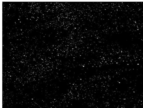
Figure 1.2: Experimental image of preferential concentration of water droplets in air (image taken from [2]).
